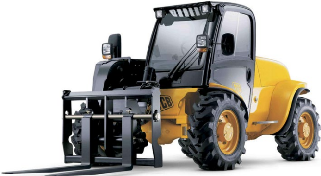
Telehandlers, like the JCB 520-40 unit shown above, are essential equipment for the operation of the Solid Waste Facility. The Town operates two telehandlers, one of which is approaching the end of its useful life.
