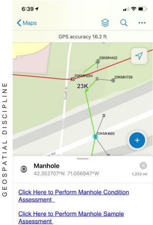
Facility ID: 23KMH693 Feature ID: 2311660660 **Owner Code:** Mass Dept of Transportation Sewer System: Storm Infiltration: Unknown Invert Elev: -999.00 .. . . -
